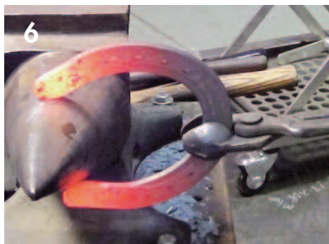
PHOTO 1: Starting on horn, using FootPro rounding hammer. PHOTO 2: Extension is nearly set. PHOTOS 3 AND 4: Heel Check is now adjusted, also on the horn. PHOTOS 5, 6 AND 7: Second heat taken to work opposite heel. PHOTO 8: Heel Check put in. PHOTO 9: Extension finished.
