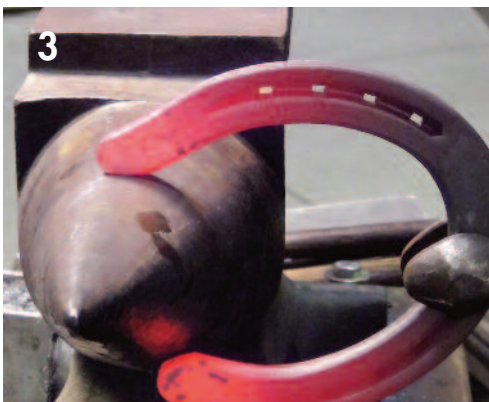
PHOTO 1: Starting on horn, using FootPro rounding hammer. PHOTO 2: Extension is nearly set. PHOTOS 3 AND 4: Heel Check is now adjusted, also on the horn. PHOTOS 5, 6 AND 7: Second heat taken to work opposite heel. PHOTO 8: Heel Check put in. PHOTO 9: Extension finished.
