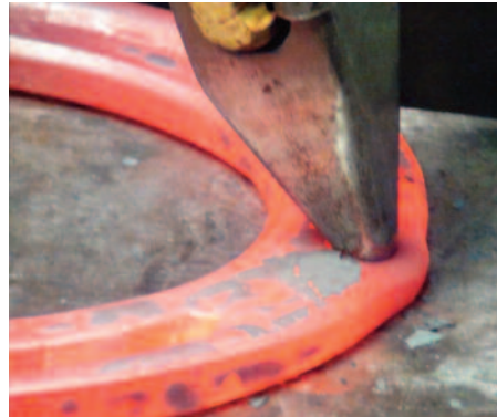
You can see the clip material begin to protrude.
