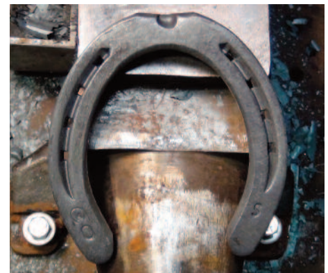
Finished clip from ground surface.
