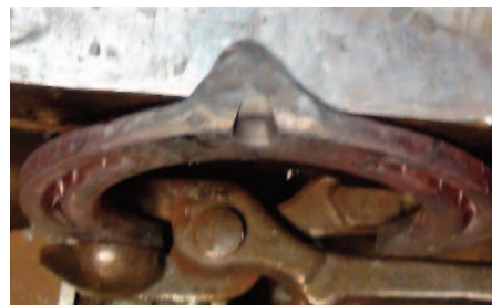
With cross tong grip, the clip is drawn on face of anvil.
