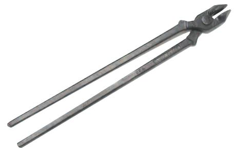
Bloom tongs set precisely for the size of stock, with parallel reins for efficient and comfortable use.
